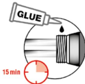
Before you apply the heating element, spread the Loctite glue (included in the set) on the middle of the thread circumference.
