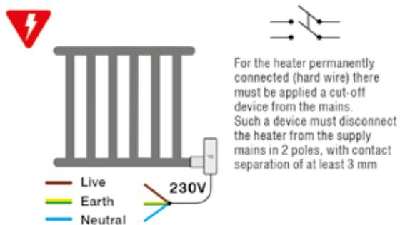
For the heater permanently connected (hard wire) there must be applied a cut-off device from the mains. Such a device must disconnect the heater from the supply mains in 2 poles, with contact separation of at least 3 mm
