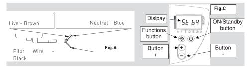
If the pilot-wire (Fig.A) is not connected, safety requires that it be insulated & in no way connected to earth
