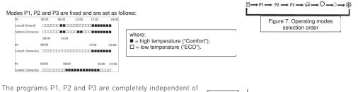
ine programs P1, P2 and P3 are completely independent of one another and can only be used one at a time. If one of these is selected (for example P3), the display appears as in **figure 8**. The flashing dash (in grey in **figure 8**) indicated the time interval currently active.
