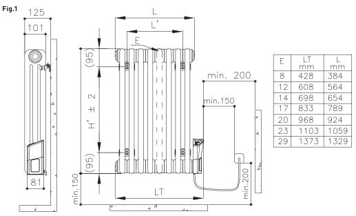
Universal Wall Brackets should be logically positioned to prevent Multi Column Electric radiators from falling away from the wall. Please refer to **3. Mark Bracket Positions & Hang Radiator (right)**
