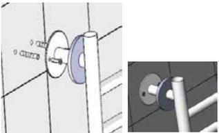
Insert long screw through mounting bracket , then screw into the plastic wall anchor with a screw driver
