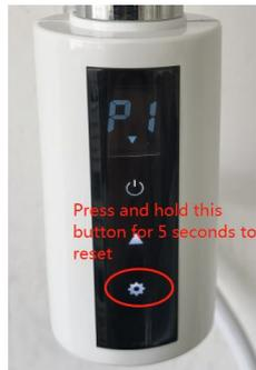
controller , coming with a sound “DI” ,the controller is now in pairing stage,and repeat the above pairing operation until the pairing work is done successfully.
